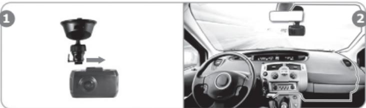
Fix the frame and the mount of the device on the windshield.
