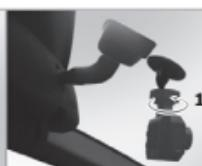
Loosen screw **1** by turning it counterclockwise. Regulate the MVR position on the mount and set the recording angle. Tighten screw **1** by turning it clockwise.
