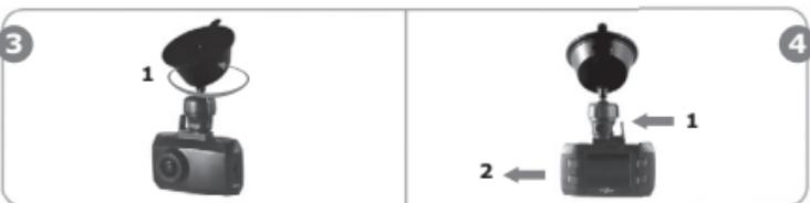
Loosen the screw **1** by turning it counterclockwise. Adjust the MVR position on the frame and set the recording angle. Tighten screw **1** by turning it clockwise.
