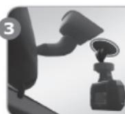
Fix the mobile video recorder on 3M scotch tape to the selected place on the windshield.
