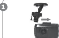
Attach the MVR frame to the 3M scotch mount.
